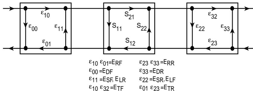
Figure 13. 8-term TRL\* error model and generalized coefficients
