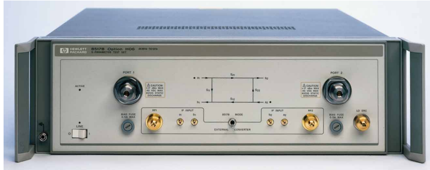
Figure 2. The HP 8517B H06 Test Set serves as the interface between the HP 8510C VNA and the OML high-frequency test modules.
