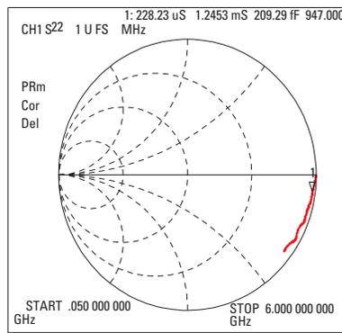
watch out for "negative" capacitance (due to long or inductive short)
