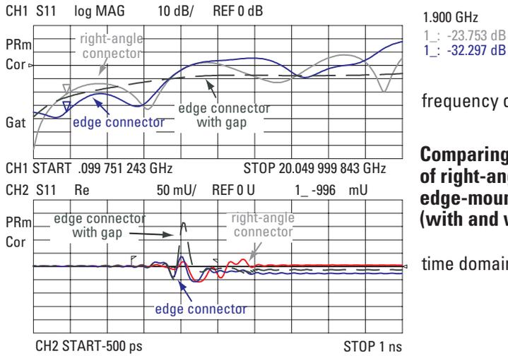
**Comparing match of right-angle and edge-mount connectors (with and without gap)**
