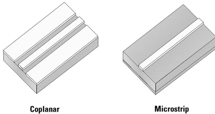
Figure 1. Types of printed circuit transmission lines
