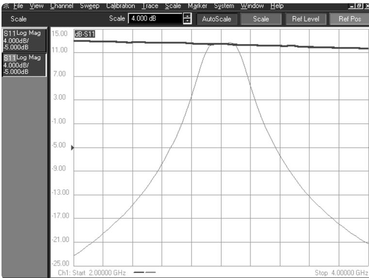
**Figure 24. Measured S21 showing the effects of embedding a virtual bandpass filter network into the measurement of a surface mount amplifier. Upper trace is the measured response of the amplifier only. Lower trace shows the response including an embedded filter network**
