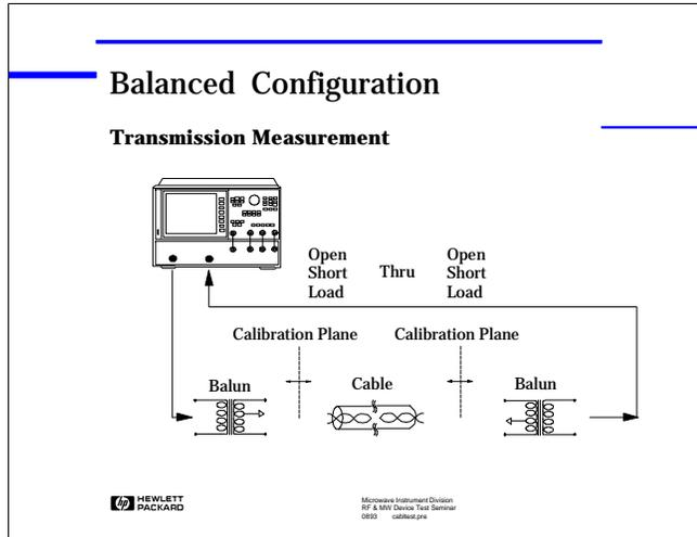
*Add another balun and a 2-port cal to perform a transmission measurement. The calibration plane is set at the end of the cable.*
