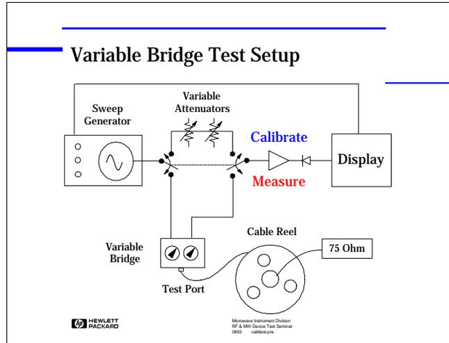
*this system. This is the grease pencil world, where you adjust an attenuator to match a level on the display.*
