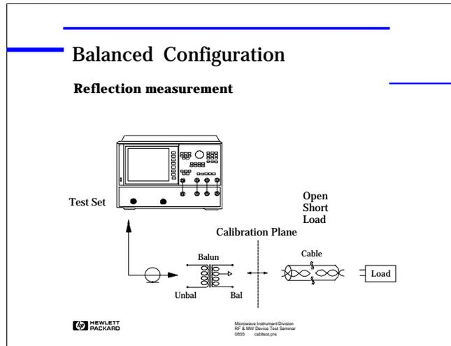
*The balun is added and the reflection measurement is performed as before. Calibration removes the measurement errors associated with the balun and system. This is true only when the twisted pair impedance does not vary. Below 1 MHz, the impedance varies widely and can cancel out any calibration.*
