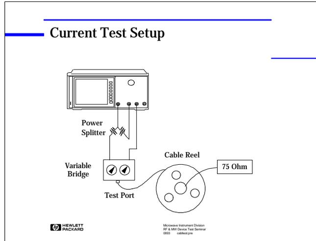
*This is the proposed system for the SCTE measurement. Better measurement but still the same problems/limitations with the variable bridge.*
