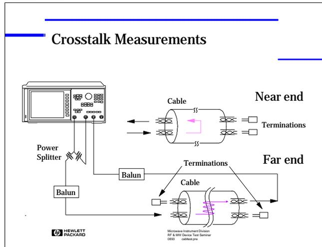
*when the induced signal levels from another pair mix with the desired signals and eventually cause disruption of transmission. This is a complicated measurement with lots of data taking and comparisons between pairs as well as switching and terminating.*
