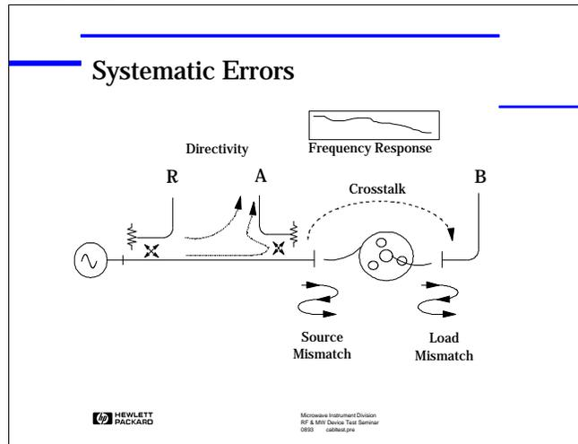
*Re-emphasizing the features of the full 2-port calibration and the errors that are removed. This slide is used in other sessions and should deserve only a brief mention of the errors.*
