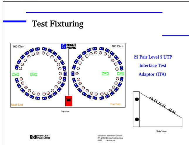
*layout allows equal lengths of pairs from the cable to the fixture.*
