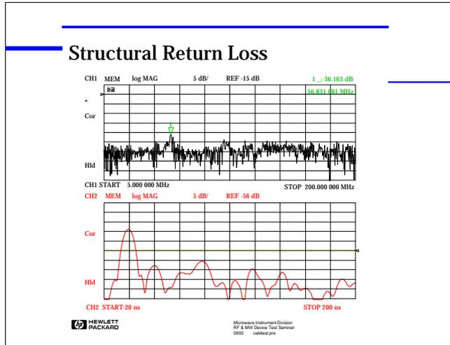
*realistic example. Note the scales for the plots and the markers. The dip in the insertion loss is just a few dB with the SRL being 15 dB or so out of spec. The old plots, one good cable and one cable after denting, are the same results as shown in the video tape. Show the video tape at this point. Be sure to point out that the dents are an attempt to simulate SRL, but from just a few dents rather than the distributed dents throughout the cable.*
