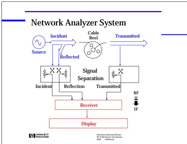
Using a network analyzer for the same measurement offers several advantages. But, first let's review the major components of the analyzer.
