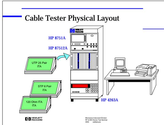
The test rack is shown here to illustrate the test equipment required and the cable connection and fixturing. A PC is used to control the operation and provide a data base of test results. Test that might require weeks manually can be accomplished in a matter of hours.
