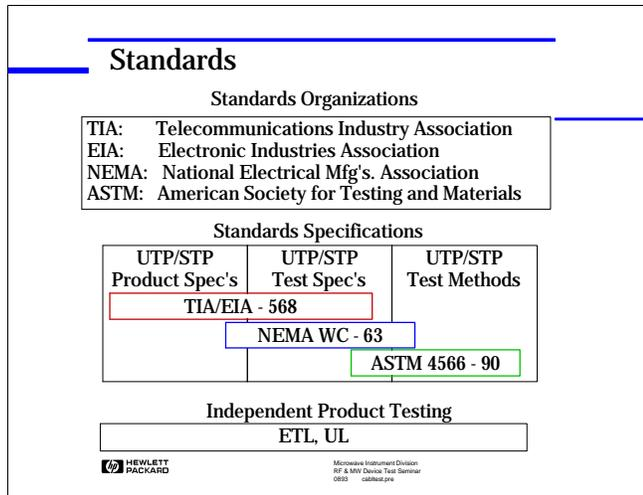
*transition. There isn't time to explain them. The latest proposal, June 93 , for TIA/EIA has some interesting new measurements, such as power sum. Each of the lines in the crosstalk measurement must be measured against all the others and then the results combined mathematically for a worst case condition. The new trends only lead more toward automation and fixturing for the measurements.*
